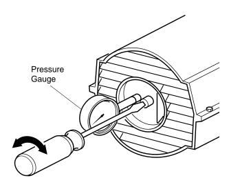
Figure 7 - Adjusting Pump Pressure
